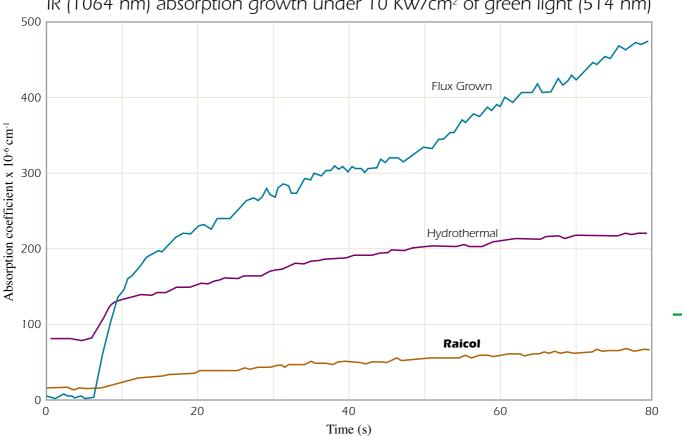
In the GRIIRA (Green Induced Infrared Absorption) test, an infrared laser beam passes through the KTP element.
