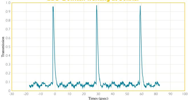
The graphs above show the behavior of RTP and BBO Q switches at high repetition rates. In particular, the BBO shows Piezoelectric ringing at 30 kHz, while the RTP Q switch shows no ringing at this frequency.
