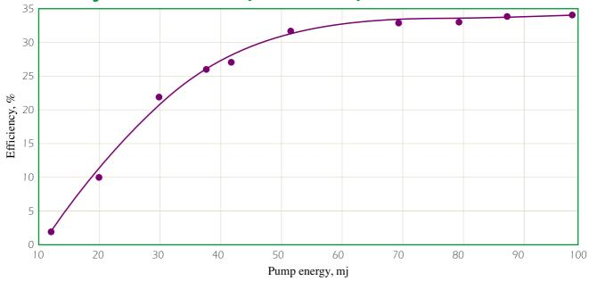
The increased efficiency of OPO conversion with a 35 mm long KTP element is shown above. Raicol can provide KTP OPO elements up to 50 mm long. Large apertures are also available.
