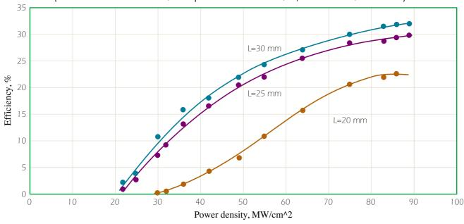
The above graph shows the increase in efficiency in OPO conversion achieved with increased KTP element length. In the past, OPO efficiency leveled off with 20 mm long elements, and actually dropped with longer elements. This was due to imperfections in the KTP elements. Raicol's crystal growth technology can provide long elements with few imperfections, which results in higher OPO efficiency.
