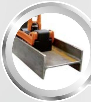
**New design allowing for the use of the magnet even between the flanges of a steel beam**
