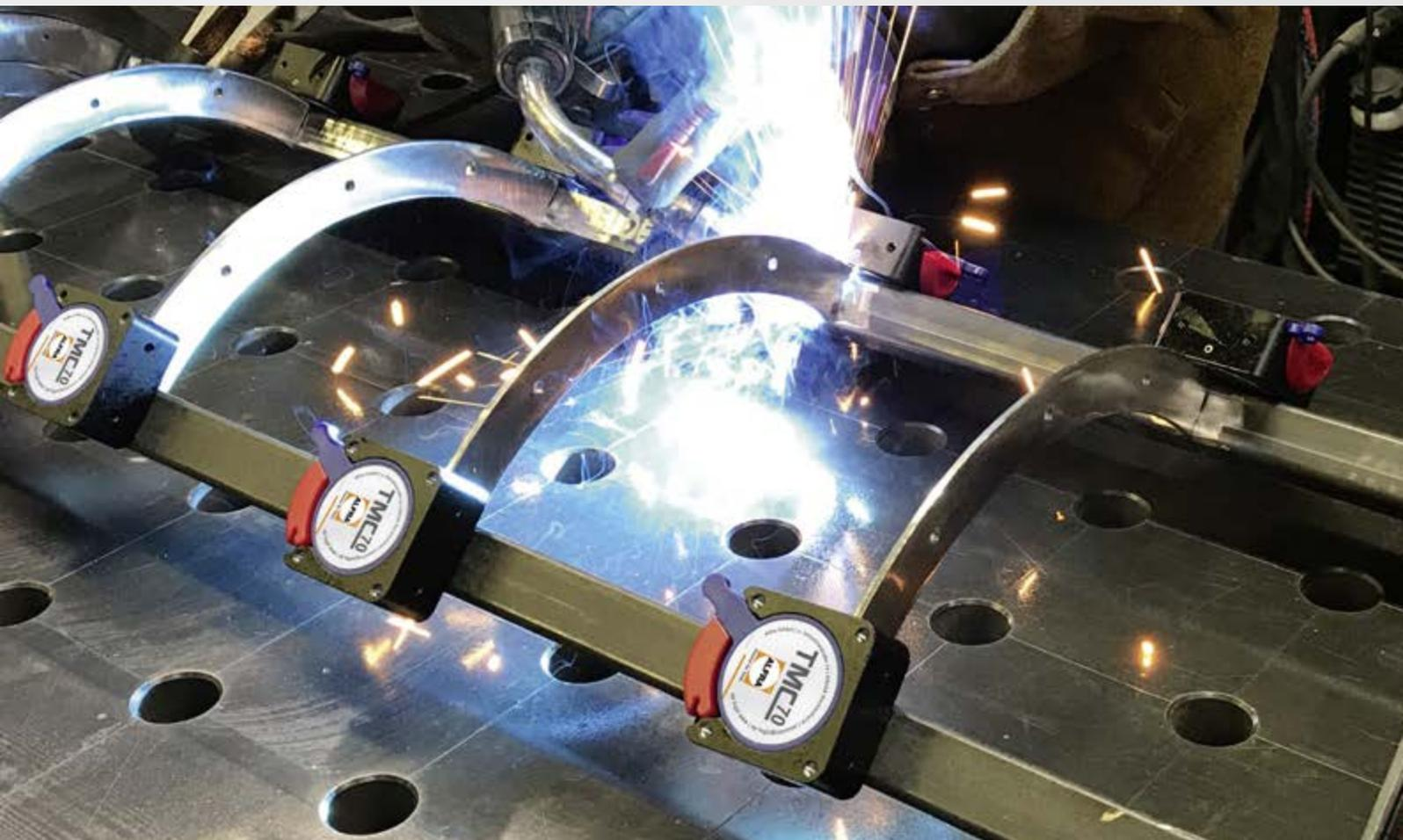
Instead of complicated clamping: The TMC 70 for easy fixing of metal parts for welding work
