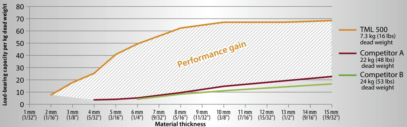
When taking the ratio of the magnets' load capacity in graph A and their dead weight into account, the hatched 'performance gain' shows the efficiency of TML magnets in contrast to their competitors.
