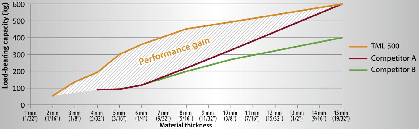
A comparison of the performance data of the TML 500 and two conventional magnets reveals how powerful the TML 500 is, especially when used on thin materials.
