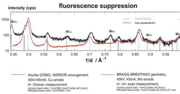
Better resolution than soller slits because of a more than two times lower angular acceptance ( $Cu K\alpha : \Delta\phi < 0.03^\circ$ )
