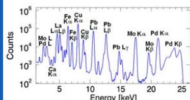
Sum spectrum of sample RF4 measured at an Eagle laboratory μ-XRF with Rh tube (20 kV) at Los Alamos National Laboratory
