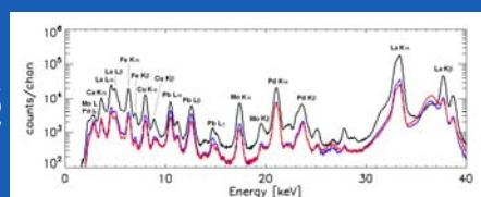
Sum spectrum of sample S10 measured at ANKA FLUO beamline (25 keV, 0.1x0.1 mm<sup>2</sup>)
