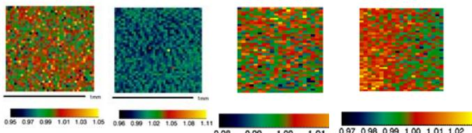
Lateral homogeneity measured by XRF μ-beam mapping (1.2x1.2 mm<sup>2</sup> with 2.8x12 µm<sup>2</sup> beam) of La and Cu, and XRF large area mapping (15x15 mm<sup>2</sup> with 0.8x0.4 mm<sup>2</sup> beam) of La and Cu (from left to right)
