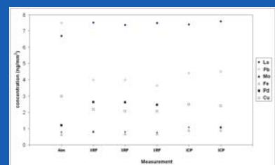
Comparison of calculated deposition amounts (Aim) and measurement results of different analysis methods (XRF and ICP-OES) for three identical reference samples (SF1, SF2, S100). Most target values were achieved and reproducible.
