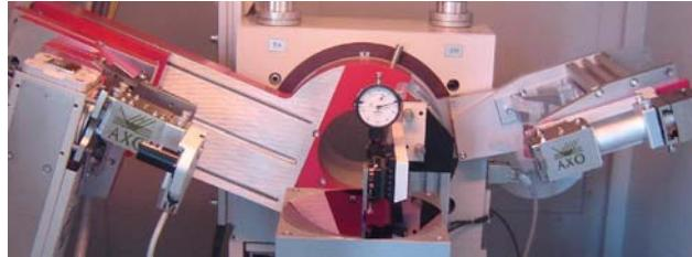
**Twin Mirror Arrangement** consisting of primary mirror with housing (left) and secondary mirror with housing, beam tube and detector slit holder (right).
