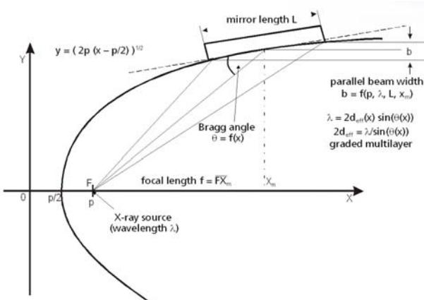
Generation of a monochromatic parallel beam in one dimension
