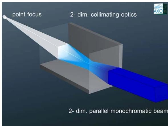
ASTIX-c: collimating geometry
