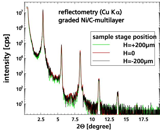
X-ray reflectometry: Independence of peak intensities and angular positions at three different stage heights
