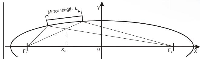
Generation of a monochromatic focusing beam in one dimension
