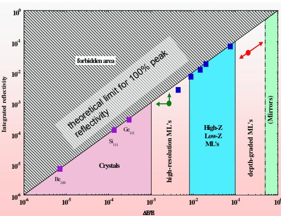
Energy resolution and divergence of hard x-ray multilayer monochromators (\*)
