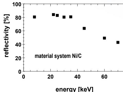
Reflectivity of a Ni/C multilayer ( $d = 4.0 \text{ nm}$ ) in the spectral range between 8 keV ... 70 keV
