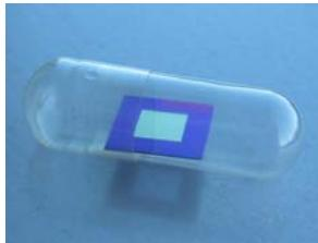
**X-ray fluorescence reference sample** with up to 7 different elements on a silicon nitride membrane (above), PEEK sample holder (below).
