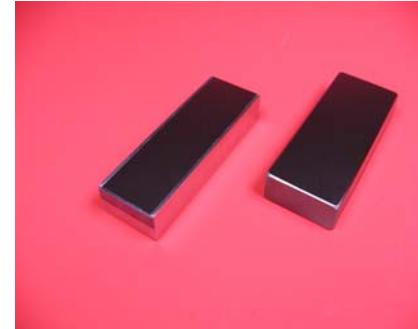
High precision 60 mm parallel beam optics on prefigured substrate (right) and on flat substrate, which are glued and bend after deposition (left)
