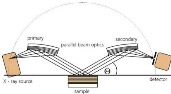
Setup of Twin Mirror Arrangement (TMA)
