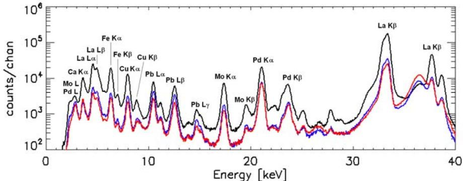
Energy spectra of three 7-element reference samples. The energy range from ~2 keV to ~40 keV is covered with peaks of comparable intensity.
