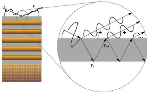
Monochromatization of X-rays by means of a nanometer multilayer stack
