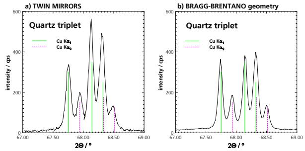
Powder diffraction measurement in the angular range of the quartz triplet in parallel beam geometry (TMA) (a) and BRAGG-BRENTANO geometry (b)
